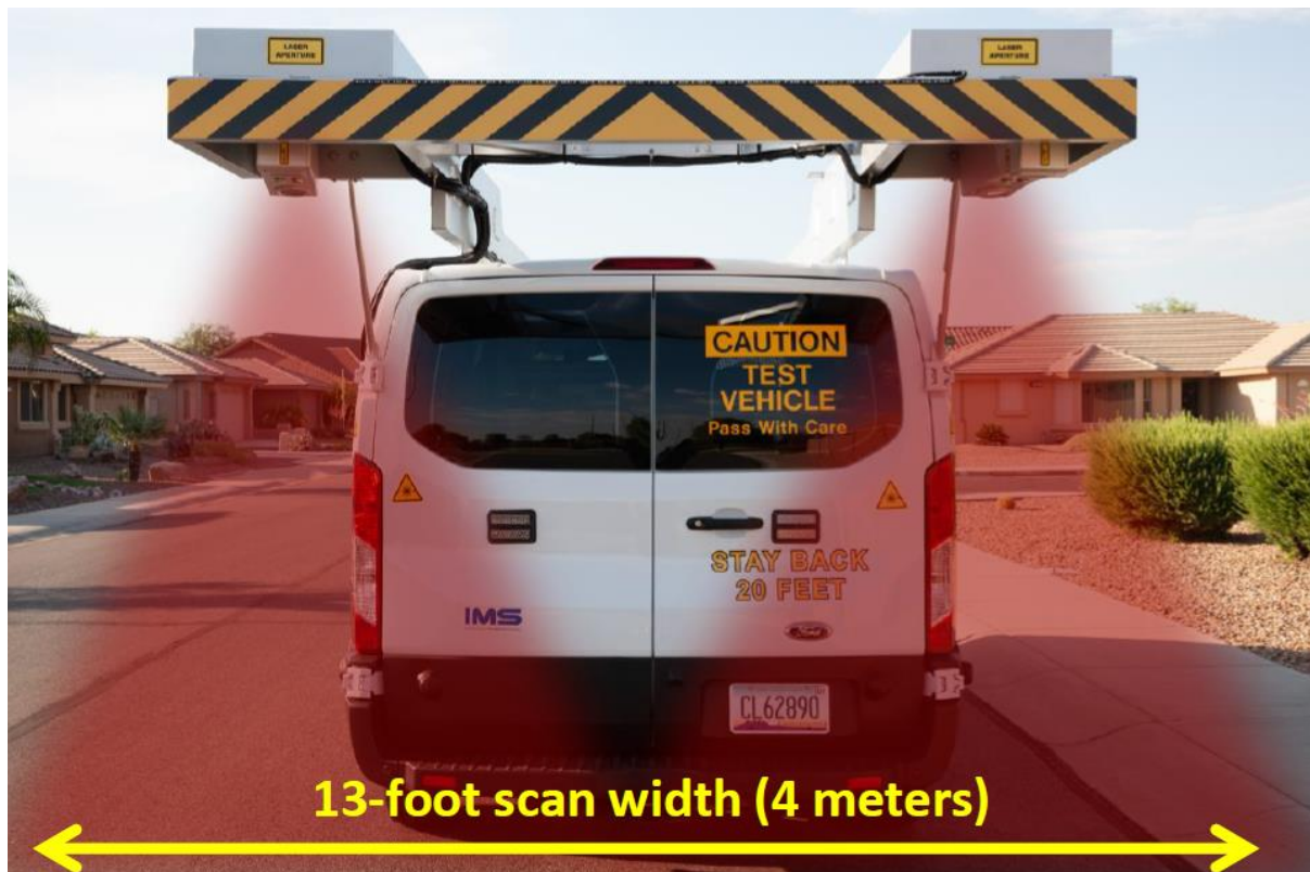
Figure 5 - RST Equipped with the 3D LCMS-2 Camera
